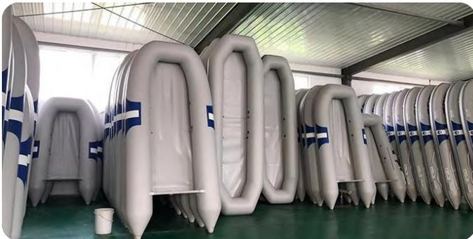
When boat is finished, we would keep boat inflated for at least 24 hours as third time testing. In addition, our quality inspector would inspect boat quality during all production period.
