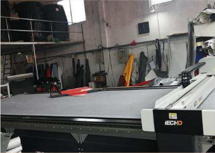
We use cutting machine for fabric cutting.
