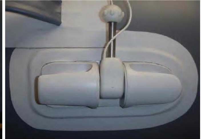
For small parts, such as oar holder, oar locker and handles. We would use extra pvc for reinforcement.
