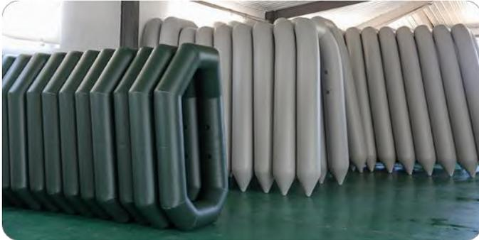
After first time testing by soap suds, we would keep boats inflated for at least 36 hours as second time air testing.
