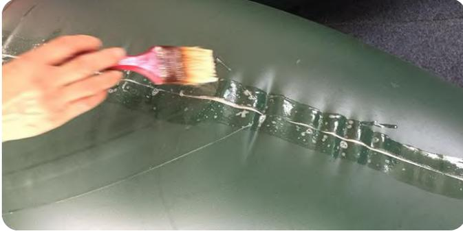
When the tube is finished. We would use soap suds to test if any air leaking.
