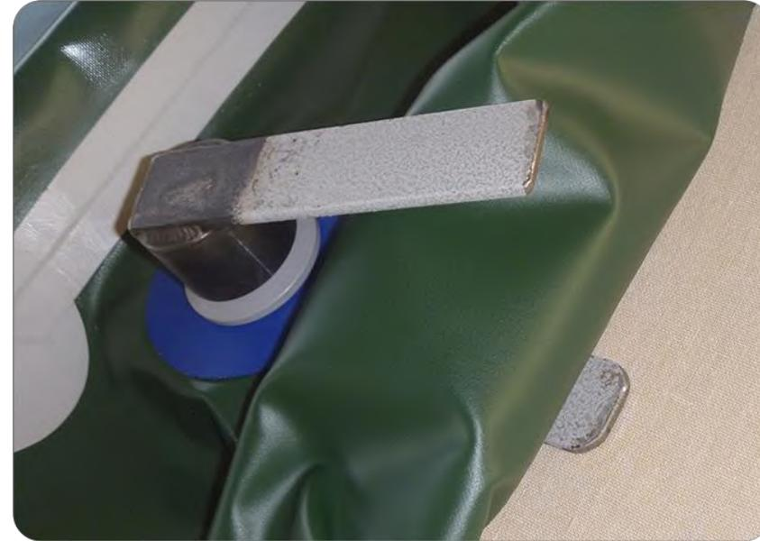
For every valve on boat, we would do testing. And use valve adaptor to tighten it and avoid any leaking.
