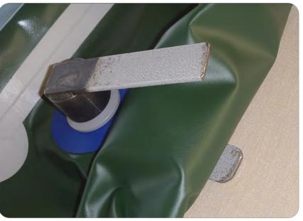
For every valve on boat, we would do testing. And use valve adaptor to tighten it and avoid any leaking.
