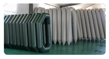
After first time testing by soap suds, we would keep boats inflated for at least 36 hours as second time air testing.
