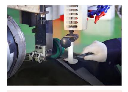
We use thermal welding machine for tube connecting.
