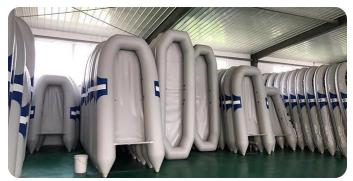
When boat is finished, we would keep boat inflated for at least 24 hours as third time testing. In addition, our quality inspector would inspect boat quality during all production period.
